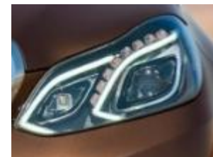
1 st vehicle with 100% LED low beam and optional camera based full-LED headlamp with glare-free high beam
